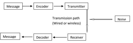
Fig.1. Outlines of a Telecommunication System
